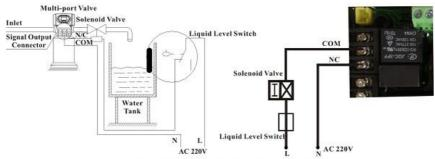
Figure 3-1 Wiring of Solenoid Valve on Outlet
