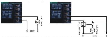
Figure 3-7 Wiring of Booster Pump on Inlet
