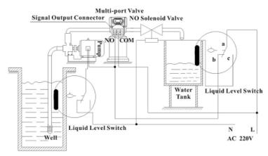
Figure 3-5 Wiring of Liquid Level Controller Controlling Inlet Pump Function:
